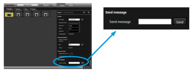
The message in the field can be sent out via the current RS-232 port. Response cannot be seen in the surface.
