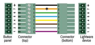
\* The 7th pin of the GPIO connector (Button panel) can be used for different functions. For more information see the Quick Start Guide of the Button panel.
