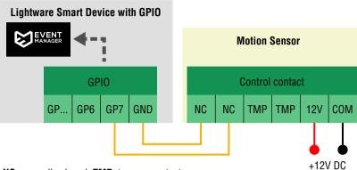
**NC**: normally closed; **TMP**: tamper contact
