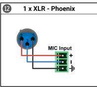
**ATTENTION!** Always check the correct wiring of the microphone cable! Never apply phantom power with unbalanced cable, because it can cause a damage!
