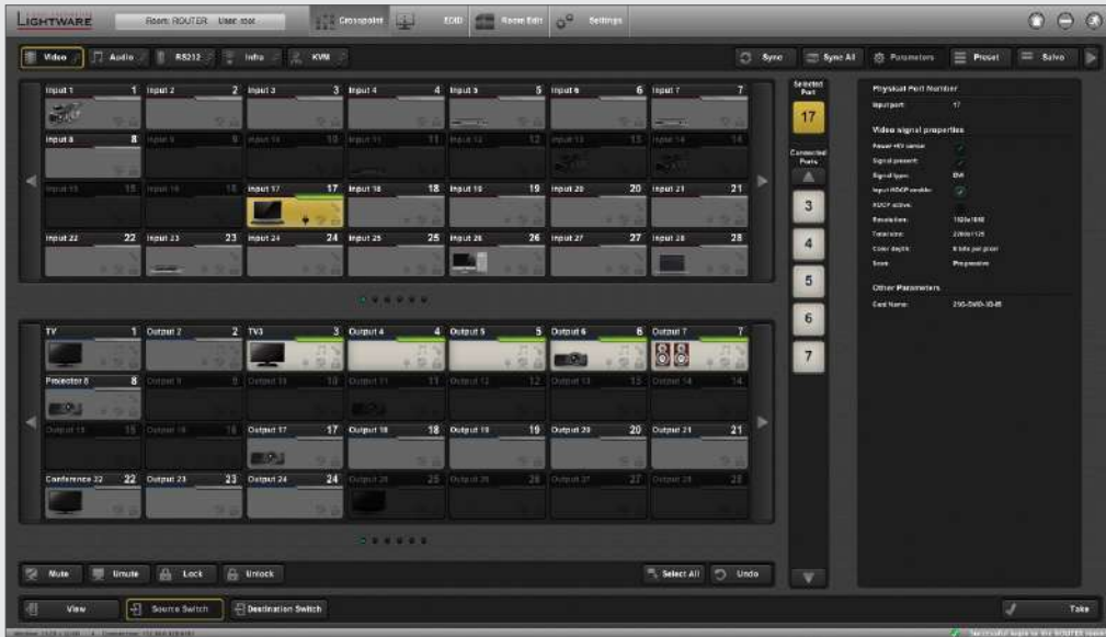
The screenshot above presents the GUI for the 25G routers. The 25G Controller is available for both Apple Macintosh and PC computers as a standalone desktop application.
