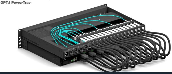
Combine an MX2-8x8-HDMI20-Audio matrix with a fully populated rack tray to create a Full 4K HDMI 2.0 optical matrix.
