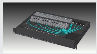
The PowerTray is a 1RU size housing accessory which can enclose up to 16 HDMI20-OPTJ-TX/RX90 units, also providing power source for every installed device. The optical fibers are connected to the four Neutrik OpticalCON Quad connectors, each carrying four signal fibers from four of the extenders. The HDMI tail cables of the extenders are accessible directly at the back of the PowerTray.
