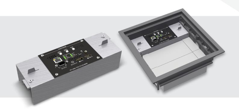
The FP-UMX-TPS-TX130-MKM Black is a flagship model in the Lightware TPS (HDBaseT™ Transmitter) product family. The device can transmit universal video, audio and control up to a 170 meter distance over a single CAT cable in dynamically changing environments such as small board rooms and classrooms. The extender was designed to handle digital and analog video and audio signals: VGA, YPrPb, HDMI 1.4 and DP 1.1 with analog stereo audio from local inputs or embedded 7.1 HBR audio.
