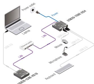
Creating a system using a PoE+ capable Ethernet switch
