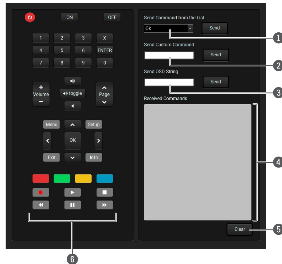
CEC control panel on the HDMI out port properties window
